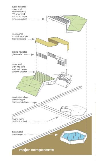
The ICE haus is fueled by biomass waste from local timber and agricultural industries. Both ice and water are stored in the cistern for summer use. A system of service trenches carries water to and from the cistern as well as heating and cooling loops to all buildings on the campus. Planted berms made from excavated earth and asphalt shelter the cistern, and create programmed micro-topographies on the otherwise flat site. Boilers and pumps are housed in an engine room visible from the Main Hall.
